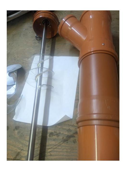
this is made from thermoplastic circles cut out with a jigsaw, softened and shaped using hot water and heat gun, then glued to the turbine shaft with silicone
